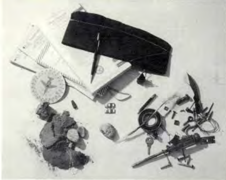
Examples of items that have ruined engines. FOD, expensive, hazardous and deleterious to mission capability, can be prevented by alert aircrew and maintenance people.
